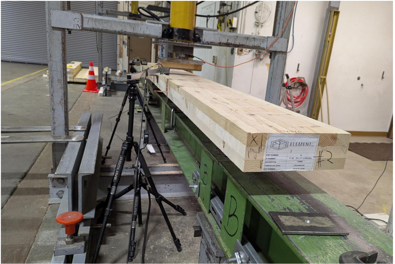
Samples of long-span cross-laminated timber made from spruce-pine-fir milled at Milan Lumber.
